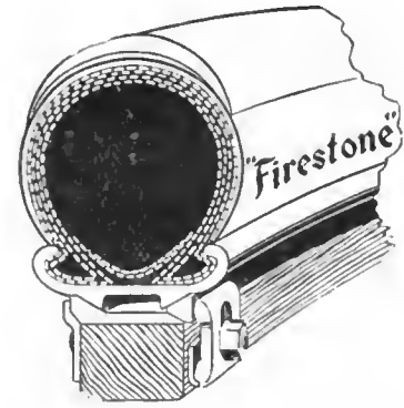
Fig. 1—Firestone demountable rims for Fords
